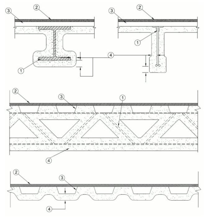
1. Steel Supports — Min W6x16 steel beam or 10K1 steel joist (See Item 4).
