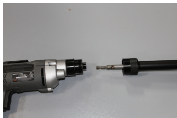
Screw the extension tube onto the screw gun adapter.
