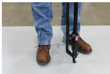
Pull the trigger to start the motor, press the footplate with constant force against the work surface. Do not remove the tool from the work until the clutch disengages and the bit stops rotating, signaling a fully driven screw. The next screw will be automatically fed into place when the tool is removed from the work. This tool has a depth-sensing clutch and will automatically disengage making a click ratcheting noise signaling a completed drive.
