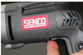
Be sure the screwdriver is operating forward (clockwise) direction. The screw will not advance and bit will be damaged otherwise.
