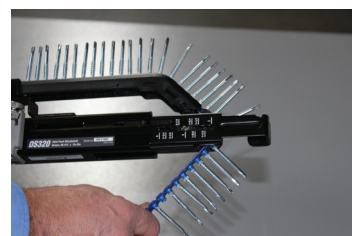
To remove the strip, pull it through the auto-feed end assembly.
