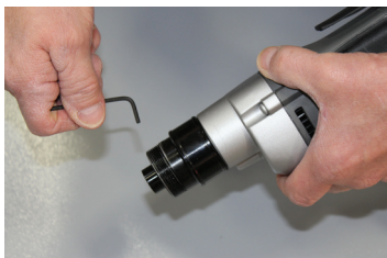
Confirm the adapter set screw is tight.
