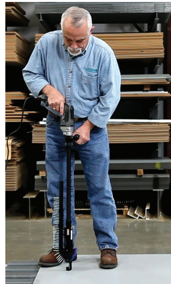
Adjust screw depth by turning the depth adjustment thumb wheel. Refer to the graphics on the tool for proper direction.
