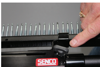
Install the auto-feed end assembly by slipping it over the top of the extension tube and tighten down with the screw adapter until snug.
