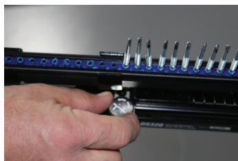
Adjust screw depth by turning the depth adjustment thumb wheel. Refer to the graphics on the tool for proper direction.
