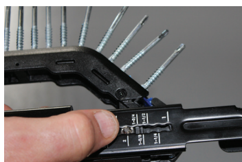
Confirm that the setting for screw length is set to 2-1/4".
