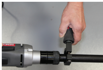
Slip drill handle over extension tube and tighten down.
