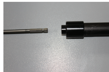
Insert bit tip into the center of rod inside the extension tube. Push down until the rod clicks into place.
